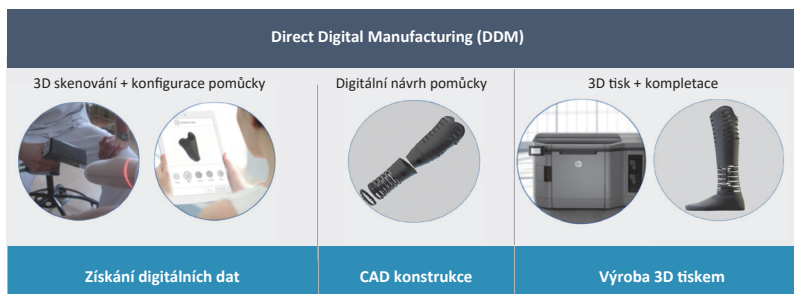
Obr. 3.17 Direct Digital Manufacturing – procesní schéma (Invent Medical Group, ČR)
